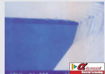
HS-HP cutting edge after cutting 1000m of Spruce
