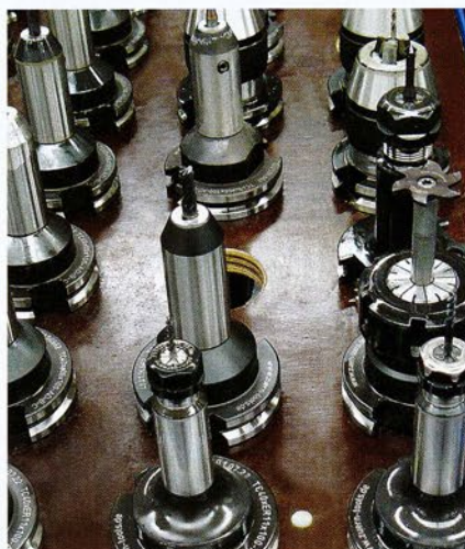
Between 20 and 25 tools are set up per tool trolley. So tooling can be assigned to non-productive times.
