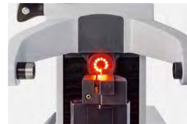
Center height measuring camera on the optics carrier with LED ring light
