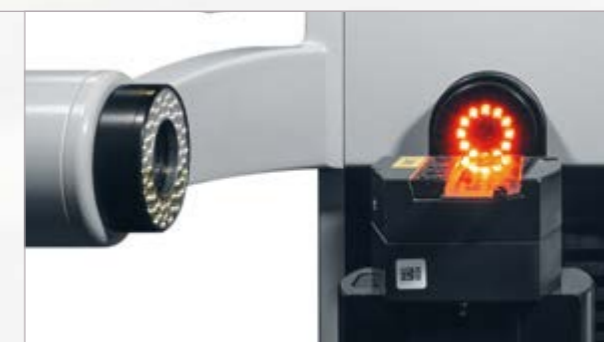
Center height measuring camera on optics carrier with LED ring light
