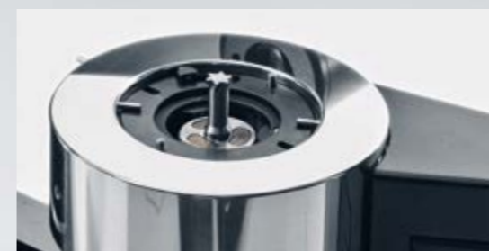
Fully automated with »tribos« The SCHUNK TRIBOS clamping unit is automatically positioned to the clamping position and returned to the starting position at the end of the clamping/unclamping process.
