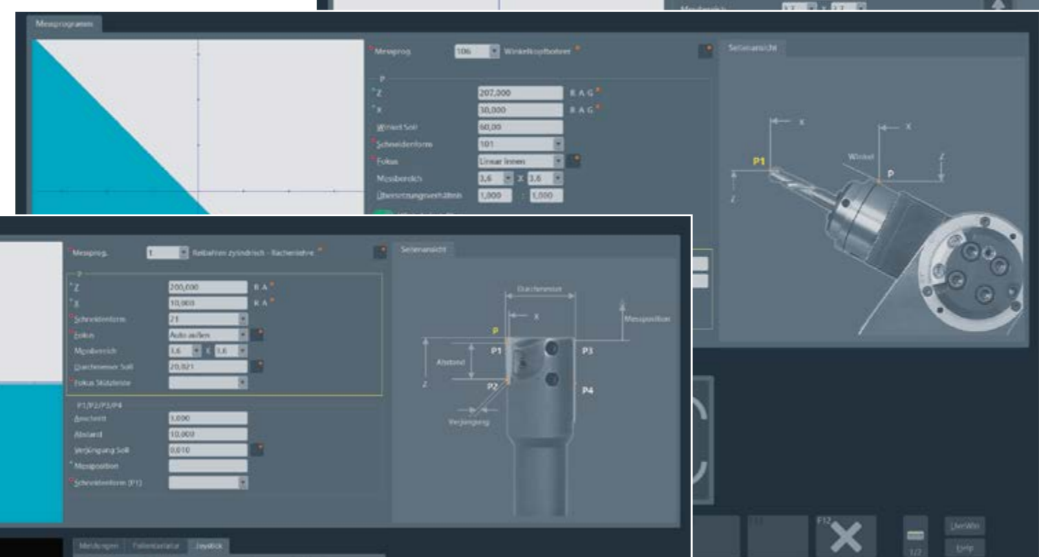
Adjustment and measurement of boring tools in angle heads. (measuring program 106)
